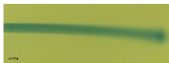
Figure 2: EBT3 film scan of a 180 MeV proton pencil beam trajectory in a PMMA phantom deflected by the transverse magnetic field.
