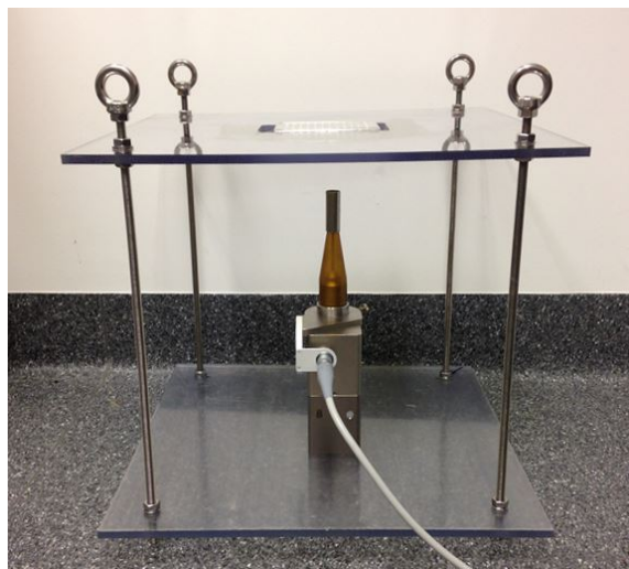
Figure 2: Cell irradiation rig with Intrabeam, collimator and 96 well cell culture plate.
