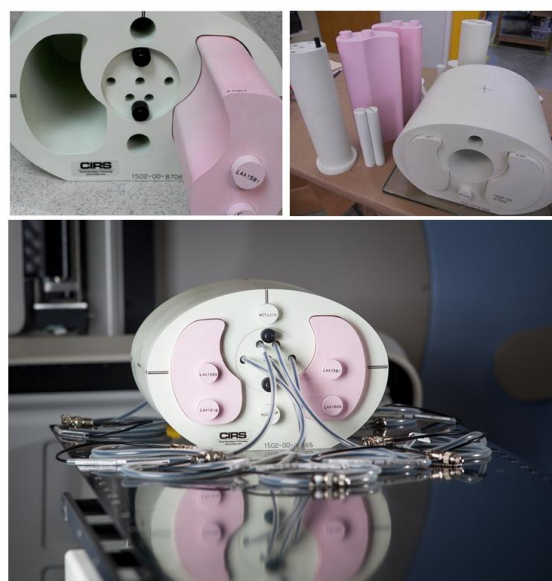
Figure 1 Images of the custom CIRS phantom for the new ACDS Level III audit, showing the removable lungs and removable central insert.
