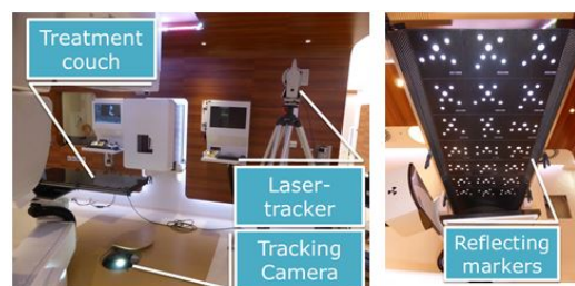
Figure 1: Setup of PPS with tracking camera and lasertracker in the treatment room is shown on the left. Pattern of reflectors on bottom side of treatment couch are on the right.
