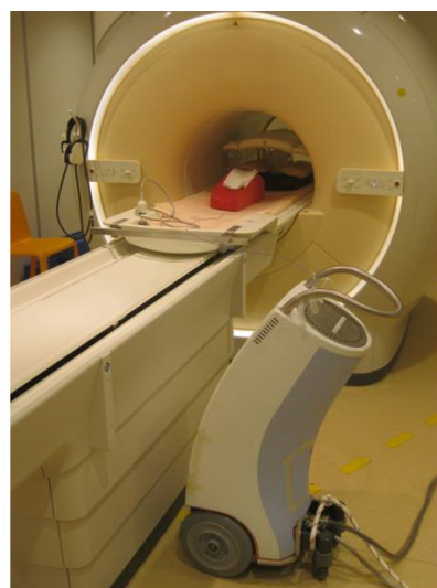
Figure 1. Experimental set-up with the prototype MR compatible afterloader placed next to the MRI scanner, a phantom placed inside the MR bore and the afterloader connected to a tube positioned in the phantom.
