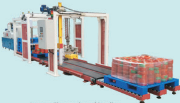
Auto coiling and stacking line
