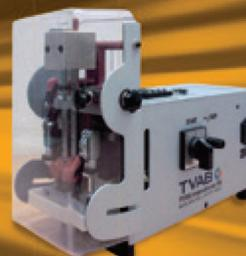
The TVAB abrasion tester is so precise that it has set the standards for ISO 6722-1. It has been designed to test the durability of cable insulation under extreme conditions and measures very specific durability variables.
