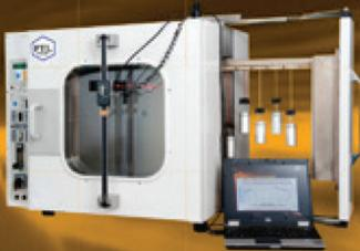
UT 6050 Hot-Set (Hot-Creep) Oven with glass observation panel and opto-electronic laser system for determination of the Hot-Set Elongation according to IEC 60811-2-1 and ICEA T28-562. Optional available with Air Flow Meter and Regulator. No compressed air required!
