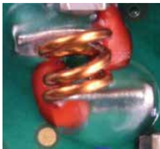
Figure 4: Pre-coating on air coil legs.
