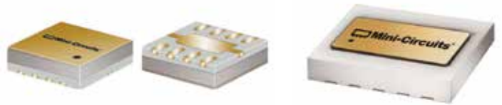
Figure 2: hermetically sealed cavity packages.
