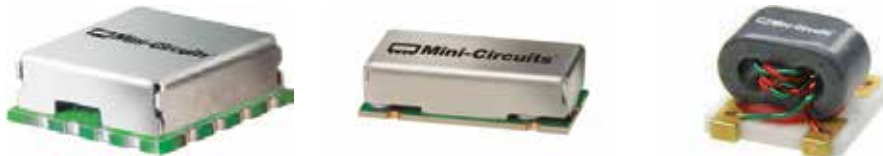
Figure 3: semi-sealed and open component assemblies
