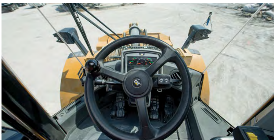
The Cat 966L comes with an improved cab with a new indicator and button layout designed to improve operator productivity and safety, new larger convex mirrors to improve visibility to the rear, as well as integrated spot mirrors to provide visibility close to both sides of the machine.
