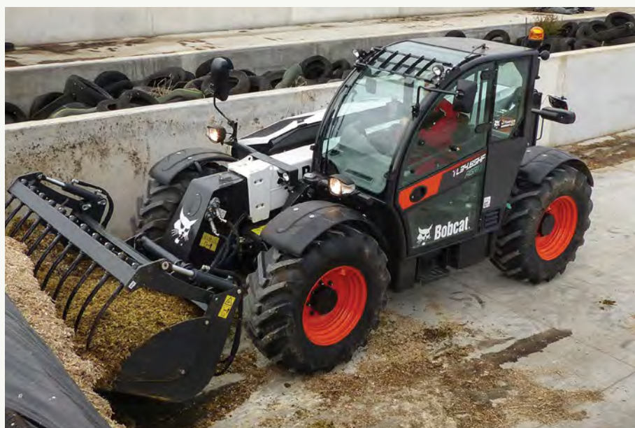
The TL34.65HF is a brand new high productivity model providing a maximum lift capacity of 3,4 t at a maximum lift height of 6,42 m.
