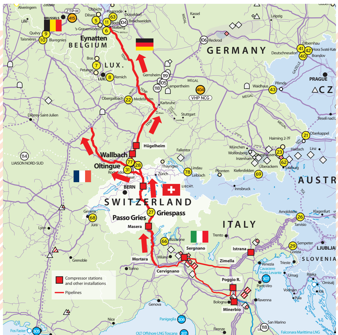
Figure 6.3: Overall schematic representation of the reverse flow projects (Source: Elaboration of SNC GRIP co-authors on ENTSOG Capacity map)
