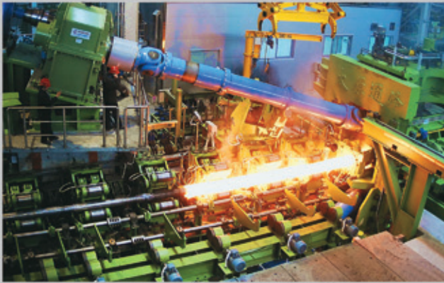
New cone type piercer for TPCO 258 line
