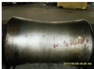
Figure 2: crack condition of forged D2 straightening roll
