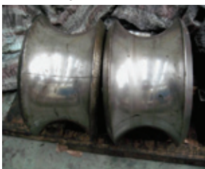
Figure 1: crack condition of forged SKD11 sizing roll
