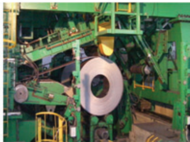
Automatic entry line
