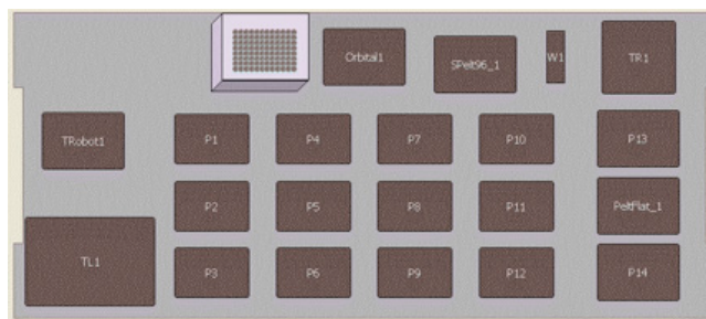
Deck configuration of the Biomek FXP Dual-Arm Multi-96 and Span 8 Liquid Handler.
