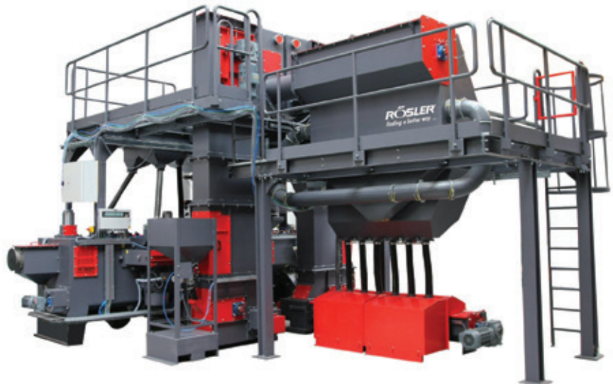
Cleaning steel bars with diameters up to 80mm
