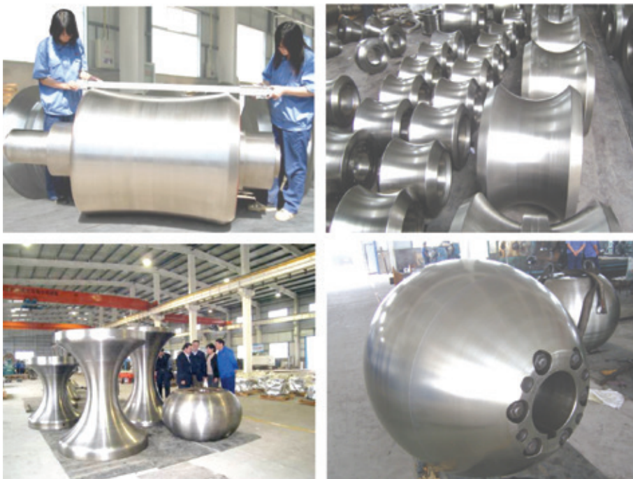
Figure 1: Straightening steel pipe roll, HFW/ERW welding pipe roll and cold roll formed steel roll
