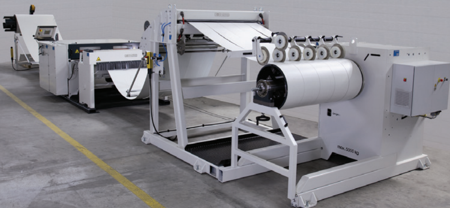
Forstner decoiling, straightening, slitting and recoiling line
