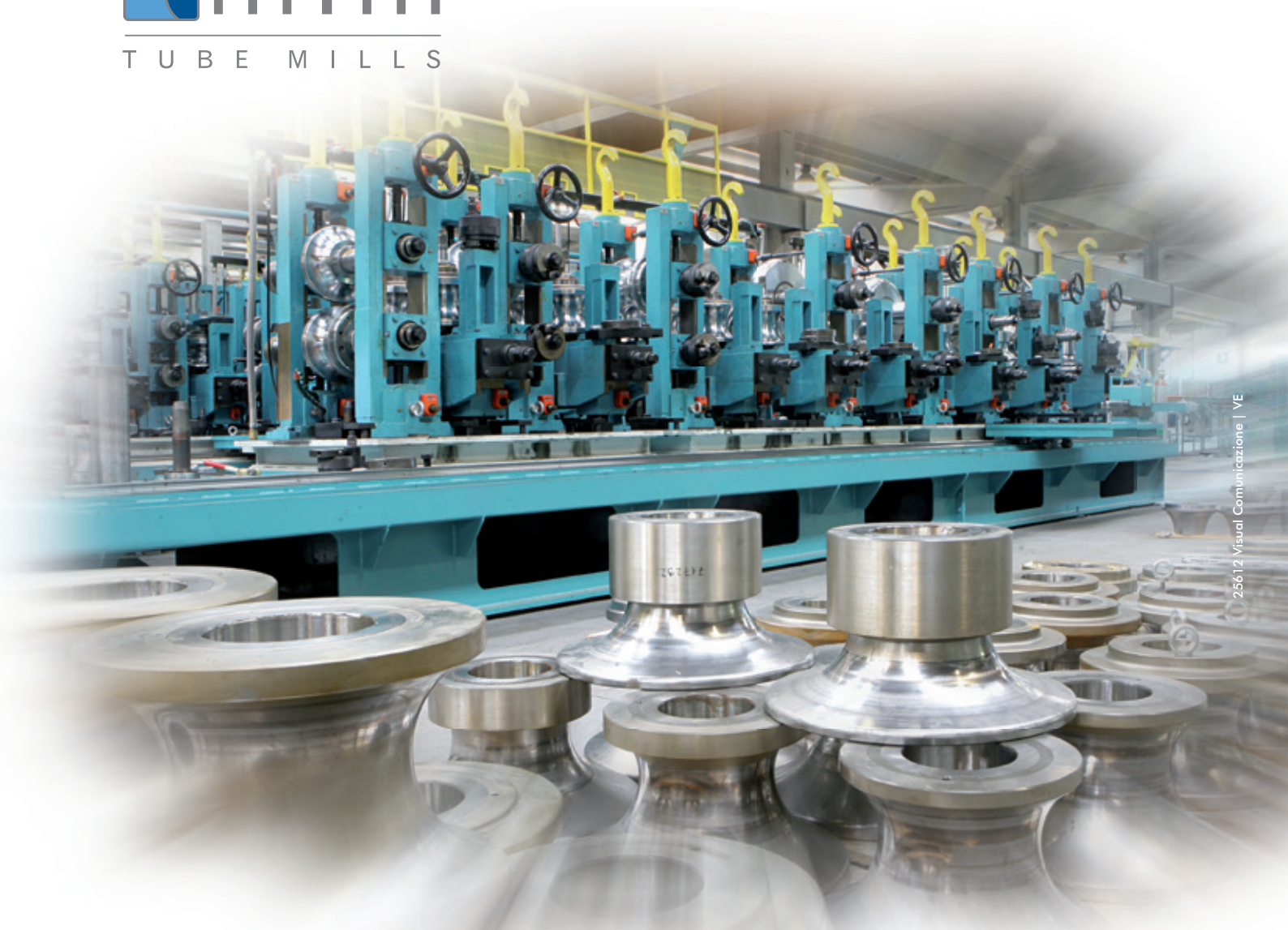
Tube forming mill and rolls for 6" tube
