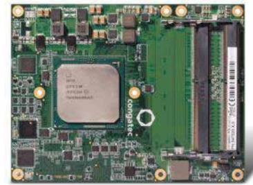
Figure 4: The new Server-on-Module from in the COM Express Type 7 specification integrates Intel Xeon processors (Codename Broadwell DE)
