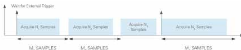
Figure 4. Example Burst Acquisition Scenario
