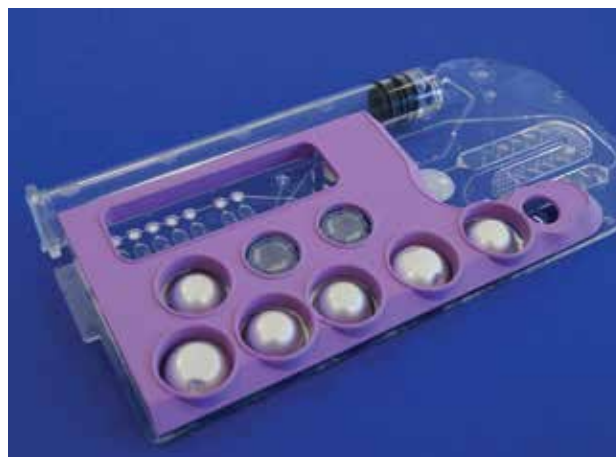
Fig 2. Integrated microfluidic device for molecular diagnostics.
