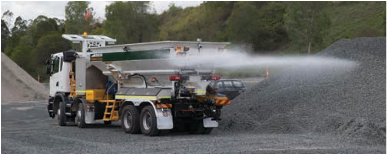
A 3 400 litre water tanker feeds the dust suppression system comprising water jets around the aggregate spouts, plus a pair of powerful jets located at the rear.
