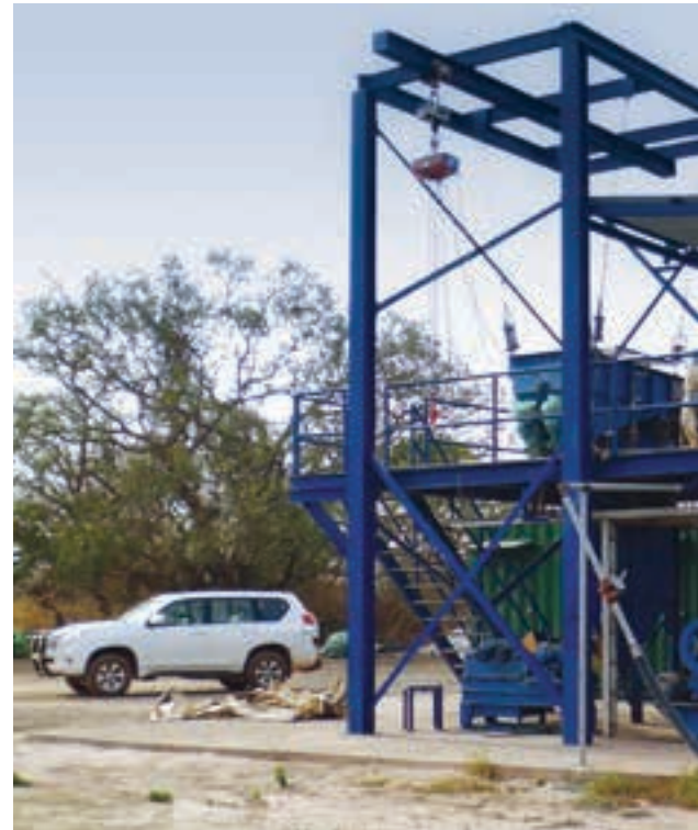
African Gold's pilot plant at the Kobada site. It has a throughput capacity of up to 2 t/h and is specifically designed for metallurgical research.
