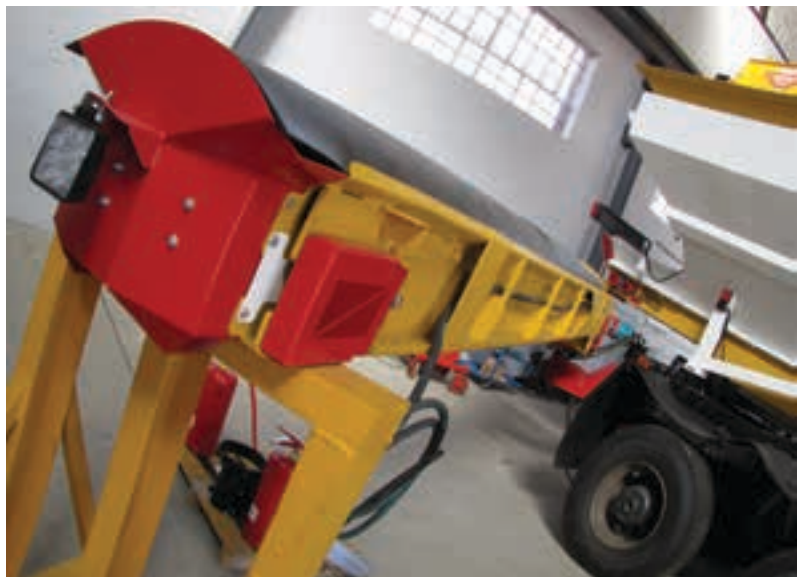
All trucks are fitted with an 8 m boom conveyor.
