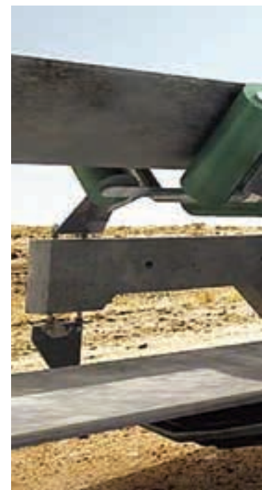
Below: Tenova TAKRAF has developed a modular overland conveyor consisting of concrete modules that can be precast on site.
