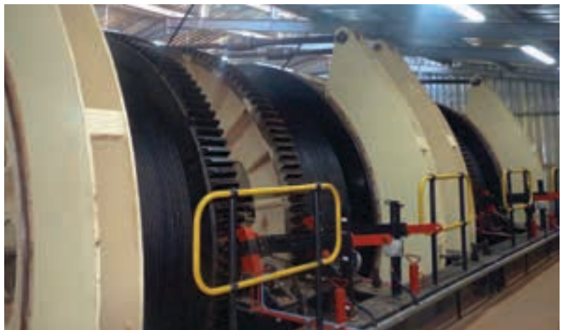
The four-drum stage winder required for the sinking phase.
