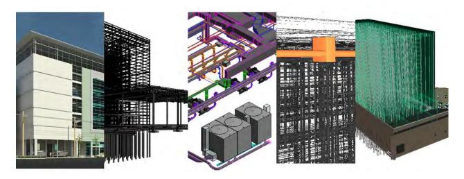
BUILDING INFORMATION MODELING OR BIM IS THE PROCESS OF DEVELOPING A VIRTUAL BUILDING MODEL THAT ALLOWS THE PROJECT TEAM TO SEE, INTERACT, ANALYZE AND COLLABORATE IN AN INTELLIGENT 3-DIMENSIONAL ENVIRONMENT. J. RAYMOND CONSTRUCTION ADOPTED THE USE OF BIM IN 2011. BENEFITS FROM BIM IMPLEMENTATION WERE IMMEDIATELY RECOGNIZED WITH A REDUCTION IN THE NUMBER OF RFIS, COSTS AND TIME DELAYS.
