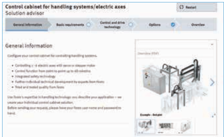
Above: The HGO (Handling Guide Online) allows the user to configure a system very quickly and then download CAD drawings.
