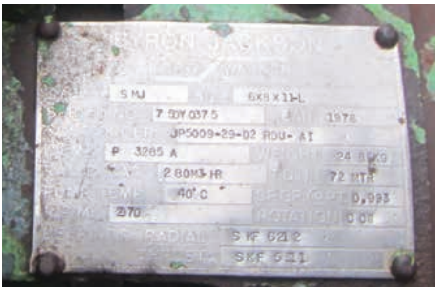
Figure 1. The nameplate of this pump shows the rated flow rate (280 m 3 /h) and total dynamic head (72 m). Note that this does not refer to the BEP of the pump, but rather the original design duty that the pump was supplied for. In many cases, the pump will be found to be operating far away from this duty, leading to major savings opportunities in energy and reliability.
