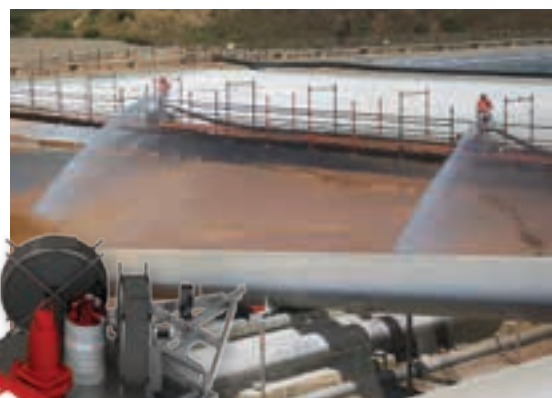
Each installation of the Slurry Blaster comes standard with a 37 kW feed pump with float, a 22 kW slurry pump for the removal of the slurry, a 200 m heavy duty layflat hose and an electric control panel.
