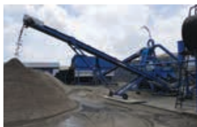
Dar es Salaam-based Estim Construction installed a CDE Combo x70 in 2014, which produces 40 t per hour of quality washed sand, whilst recycling up to 90% of the wastewater.
