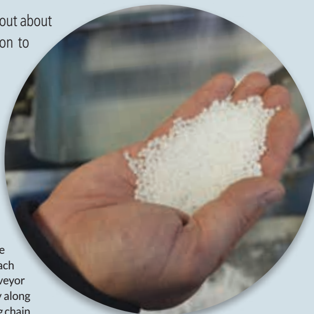
Sasol's Wax's products, such as these wax beads, are derived from natural gas and offer a combination of high melting points, low viscosity and excellent hardness, even at elevated temperatures.
