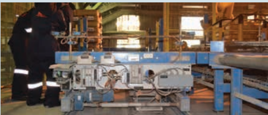
A loop of line cable on the floor, covered by installation plates between the rails of the transverse trolleys, carries the medium frequency (25 kHz) energising current.
