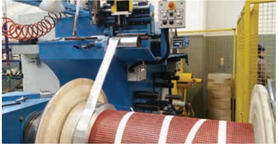
For CRTs, instead of rolling transformer wire onto a cotton-reel-like core, flat foil windings are used.
