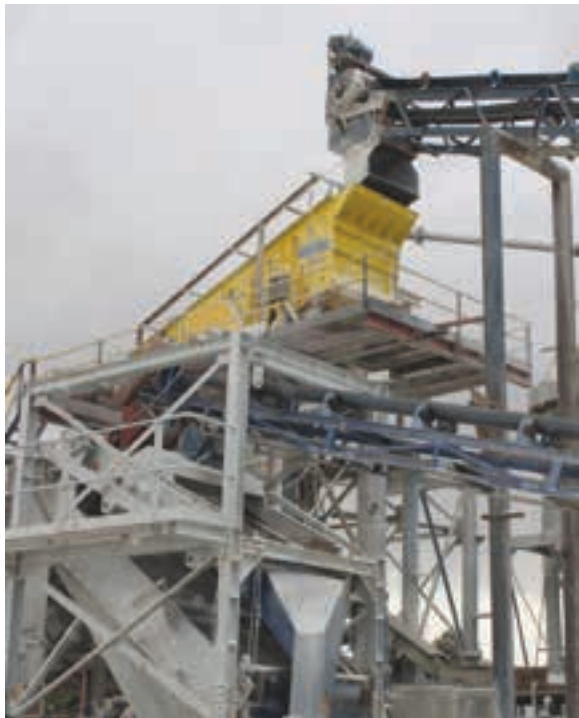
A Trio TIO5162 double deck inclined screen.
