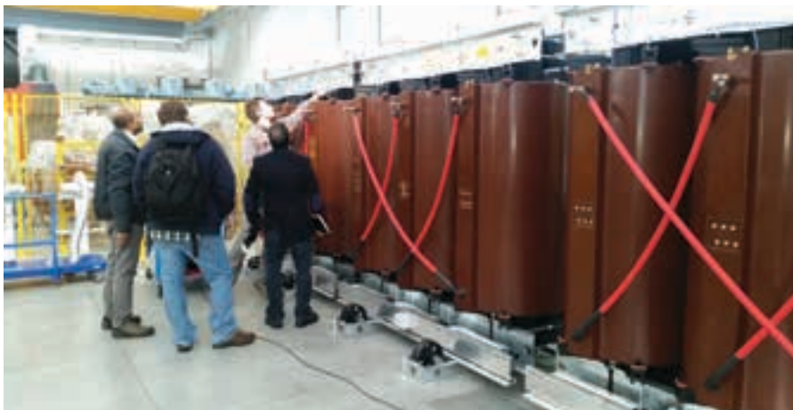
GreenErgi can offer 11, 22 and 33 kV cast resin transformers, with the largest supplied to date in South Africa being a 5.0 MVA unit for the Stortemelk Hydro plant near Clarens.
