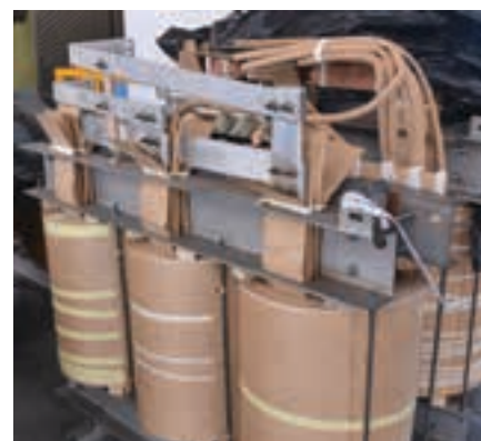
WEG Transformers has successfully manufactured thousands of transformers with aluminium windings.
