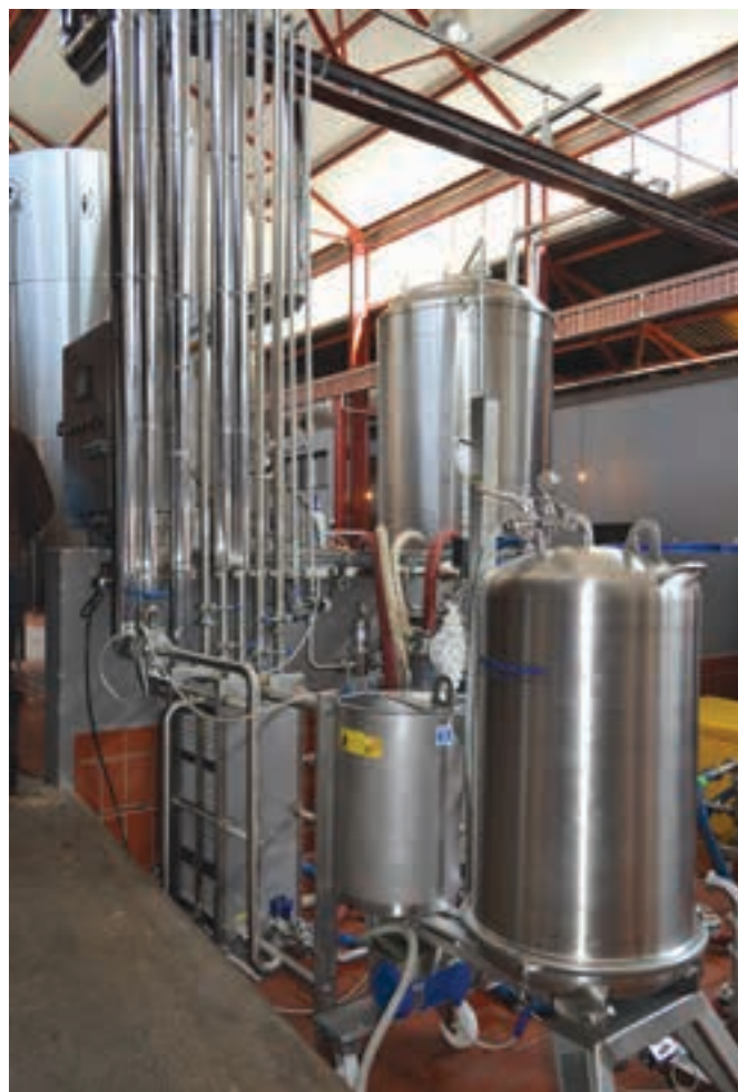
Left: For fermentation followed by maturation, Mad Giant currently has several 3 000 ℓ tanks and a few 9 000 ℓ tanks that can take three batches of any brew. Right: A clean in place network ensures that every tank can be cleaned between brew batches. In keeping with the modern environmentally aware approach, the chemicals used are recovered, where possible, for reuse.
