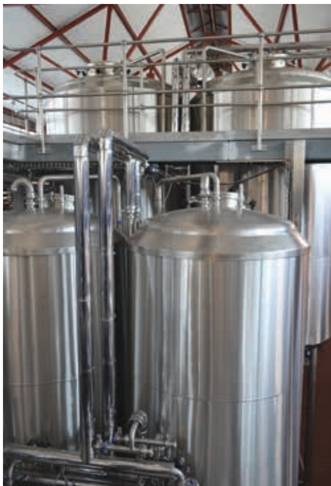
Left: For fermentation followed by maturation, Mad Giant currently has several 3 000 ℓ tanks and a few 9 000 ℓ tanks that can take three batches of any brew. Right: A clean in place network ensures that every tank can be cleaned between brew batches. In keeping with the modern environmentally aware approach, the chemicals used are recovered, where possible, for reuse.
