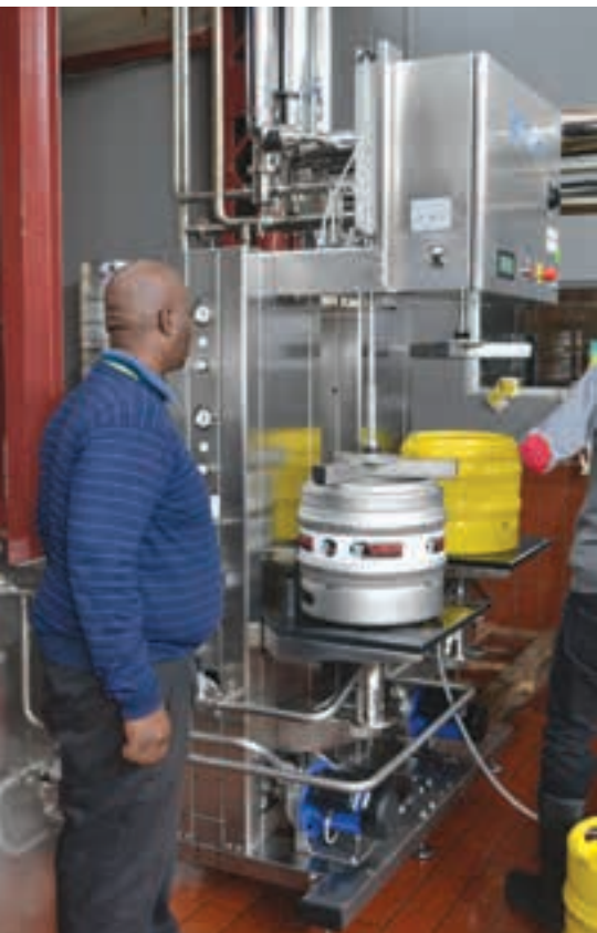
Kegs are first washed with steam. Then CO 2 is used to push all the air out before the keg is filled with beer and then pressurised using CO 2 .
