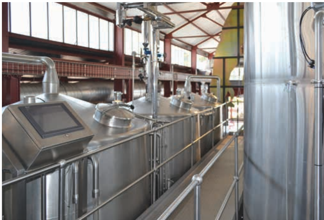
The mash tun, where the malt starch is converted to sugar, the hops kettle and associated pre-fermentation tanks where craft beer is made in 3 000 l batches.
