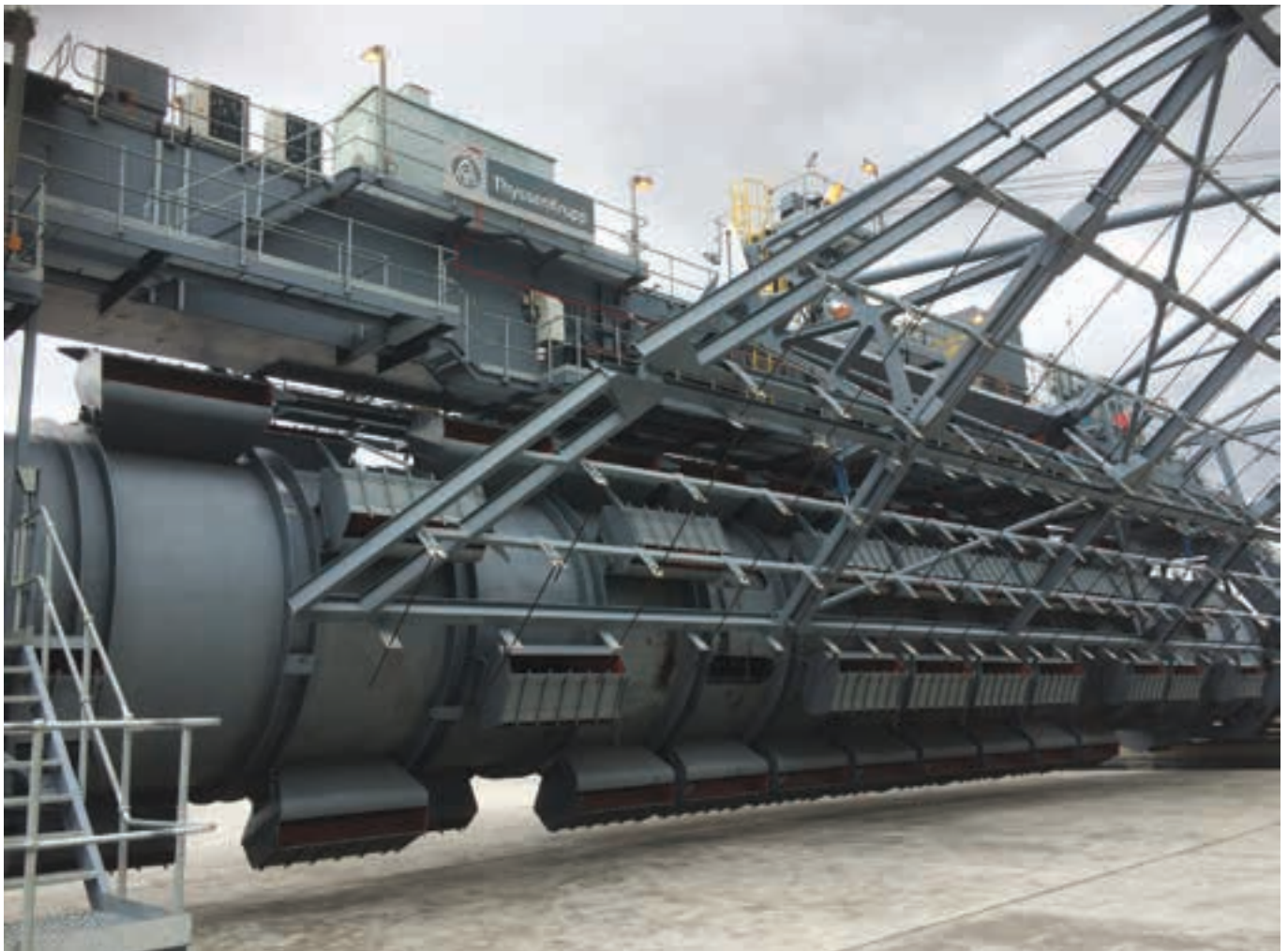
The reciprocating movement of the rakes on thyssenKrupp drum reclaimers is achieved using a single through rod cylinder with a 2.0 m stroke on each rake.
