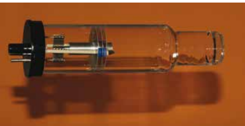
Figure 1: Flame AAS, which incorporates a hollow cathode tube, for years has been the hot choice in wear element analysis. But the increasing affordability of advanced, high-productivity ICP-OES casts a brighter light on AAS disadvantages.
