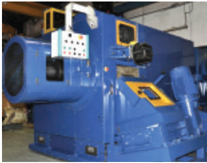
▲ Feed side of a Holton HC4000 extruder
