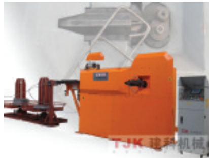
▲ 2D bending with TJK's new stirrup bender
