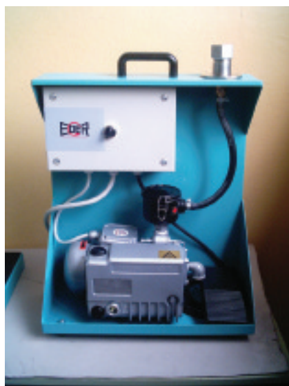
▲ Eder's VDSU vacuum drawing die suction unit
