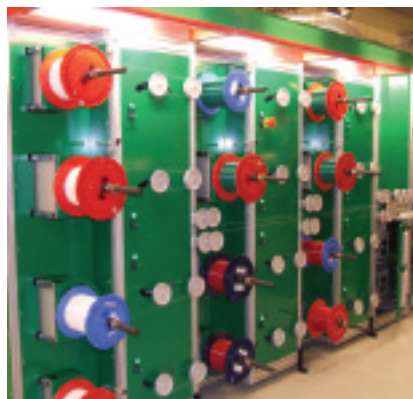
▲ The ComRIB fibre ribboning line
