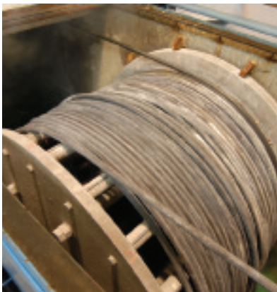
▲ Rod undergoing phosphatisation
