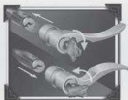
Rotate key back, remove key and cylinder. Reverse levers. Place cylinder in other lever.
