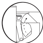
Latch retention hold is in the top latch. Retainer is released when it engages the strike.
