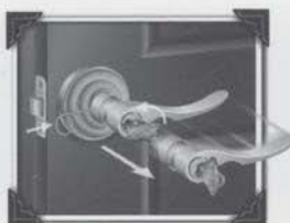
Insert key into outside lever - rotate 90°. Remove with release pin.
