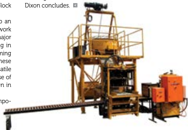
The hydraulic paving and blockmaking machine.
