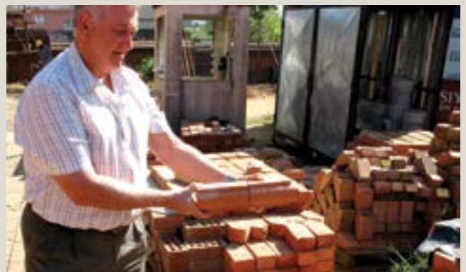
Pat Moon inspects the various types of specials and holding the concave/convex stretcher and corner brick.
