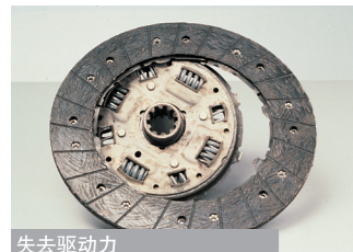
失去驱动力 Gear Loss of Drive
