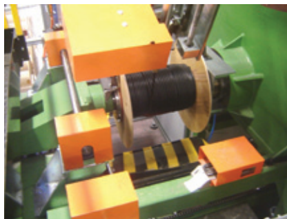
▲ The spooling phase in the new PS630/15 2B
