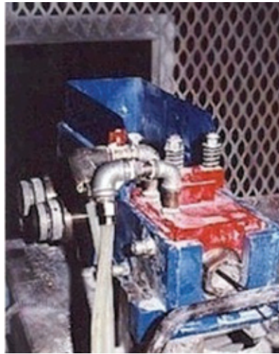
▲ Rod coating and lubrication by LVC/PDH system
