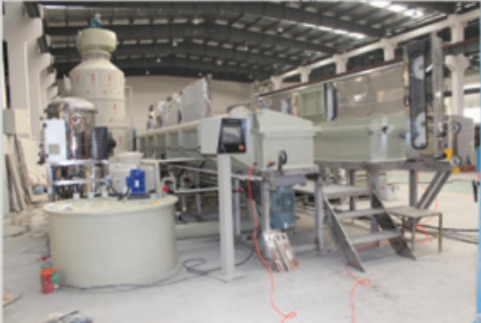
Electrolytic tinning plant (waste water free)
