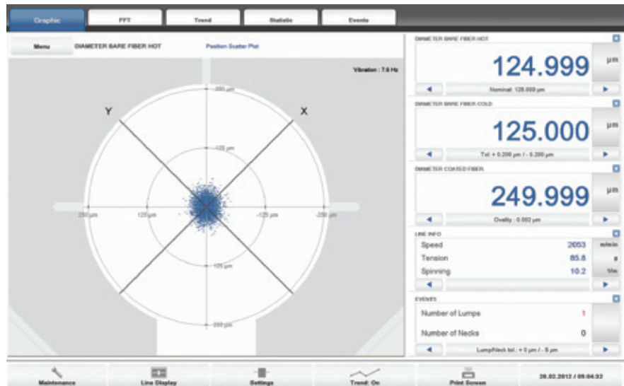
▲ Production data of the Fibre Series 6000 are visualised at the processor system Fibre Ecocontrol
