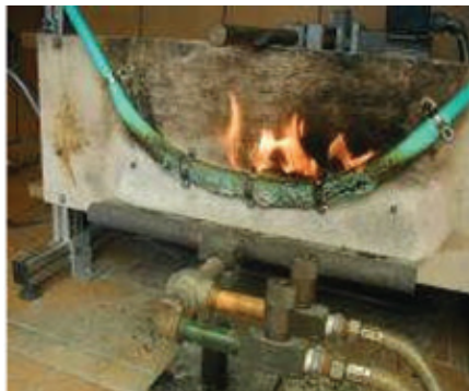
▲ Picture 2: IEC 60331-25 fire test
