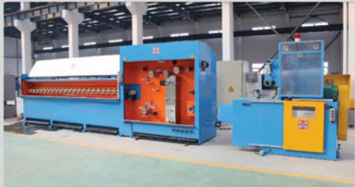
Multi-wire drawing machine with continuous annealer
