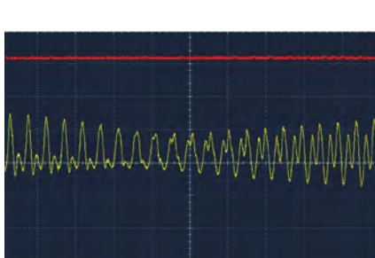
SM Oscillogram 7 Oscillogram 7. 4 x 5 W non-compliant LEDs voltage and current - direct mains (no dimmer). Horizontal: 10 us/div. LED voltage (red - 100 V/div), LED current (yellow - 0.2 A/div).
