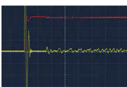
SM Oscillogram 8 Oscillogram 8. 4 x 5 W non-compliant LEDs voltage and current - startup (no dimmer). Horizontal: 10 us/div. LED voltage (red - 100 V/div), LED current (yellow - 1 A/div).
