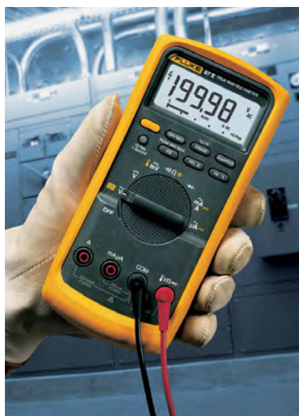
CAT ratings can be found between the input jacks on most tools
