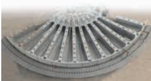
A trial assembly of the discharge system can be done on a steel jig if this is a request from the customer. This ensures fitment will be correct during the installation.
