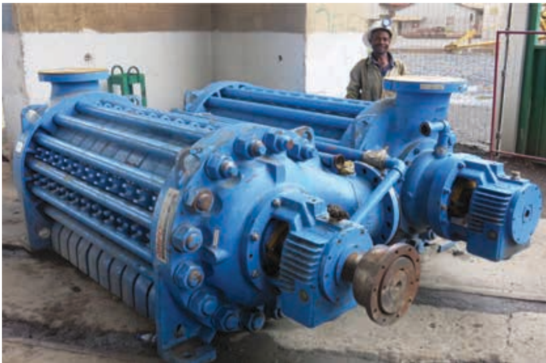
Two of three new high-volume Grifo pumps to be installed at the main pumping station 1 210 m below surface (photo: Ivanhoe).
