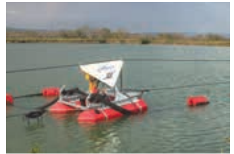
The innovative SlurrySucker dredge unit is capable of extracting high tonnages of silt and built-up sediments at a fraction of the cost required to shut down downstream and upstream processes.
