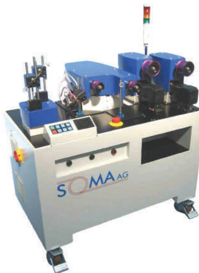
▲ USP 1000.2 – the modular rewinding solution for bonding and other ultra fine wires
