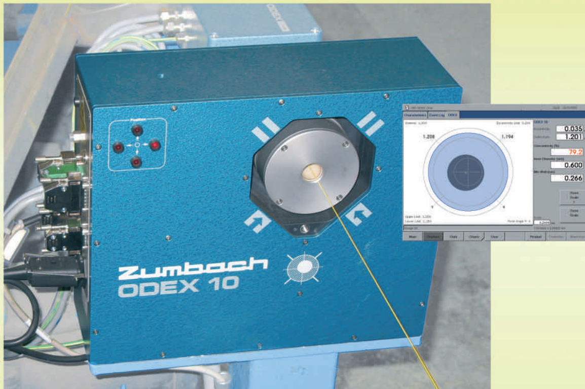
ODEX® 10 measuring unit in a extrusion line for Cat. 5, 6, ... cables.
