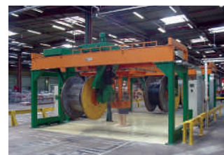
▲ Pay-off 2600 and take-up 2600 with 'U cycle' for empty drums and filled drums
