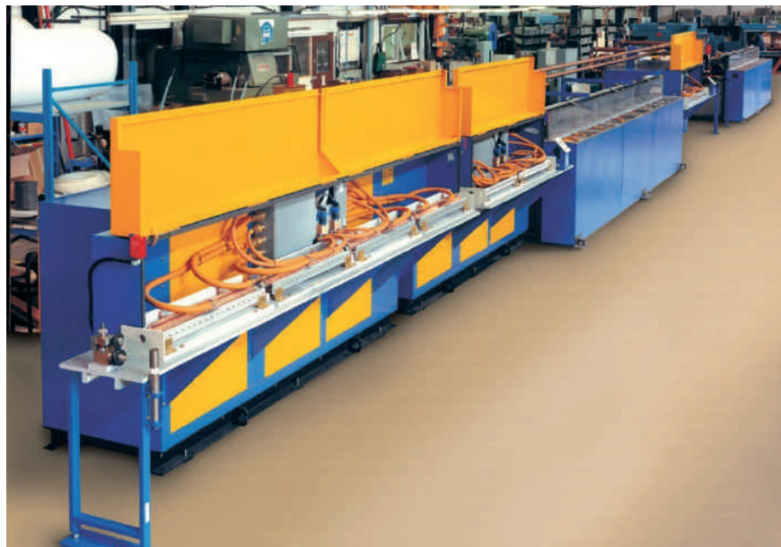
▼ Harden and Temper process wire line
