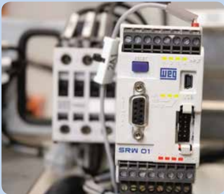
Designed for use with power supplies from 24 to 220 Vac/dc, the WEG SRW01 has a facility, if selected, to monitor voltage up to 690 V ac and measure current from 0.25 A up to 840 A.
