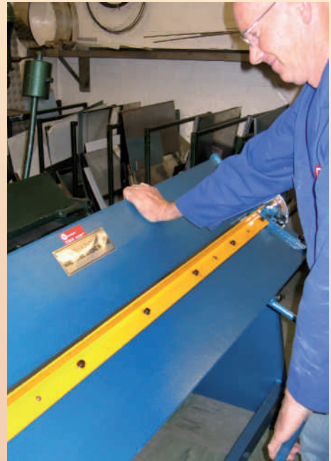
▲ The new machine will allow RG Attachments to form a variety of shapes from sheet metal
