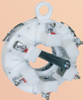
▲ UMAC Z50 Scanner with 6 measuring points (same model is also available for 4 point measurement)
