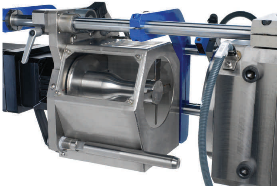
▲ The new quantec kneader from Buss incorporates a newly developed cutting device to ensure PVC pieces of uniform size
