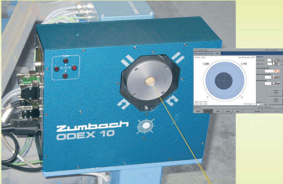
ODEX® 10 measuring unit in a extrusion line for Cat. 5, 6, ... cables.
