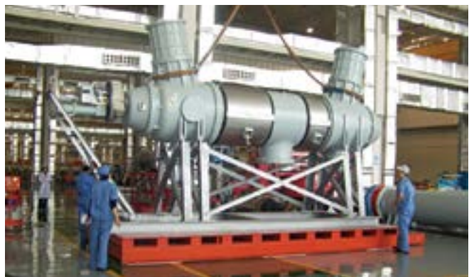
Large platform with bearers to aid forklift loading
