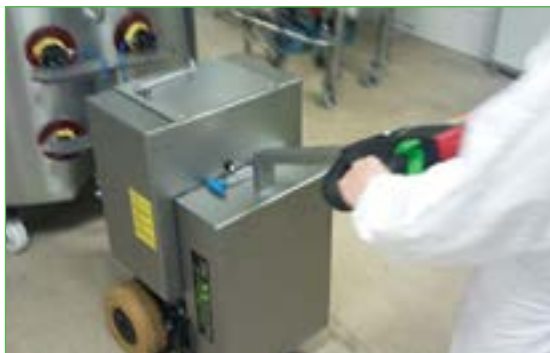
Shown with optional vacuum pad hitch
