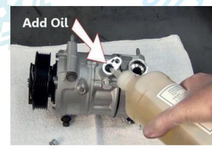
amount of oil 1-2fl oz unless GMA6/YORK (replacement compressors do not always come with oil charge!). Be careful not to over tighten the drain/fill plug as you will strip the thread! You must not over oil charge the system!
