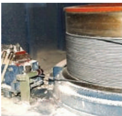
▲ Rod/wire dry coating by LVC/PDH system, in a 0.88°C application
