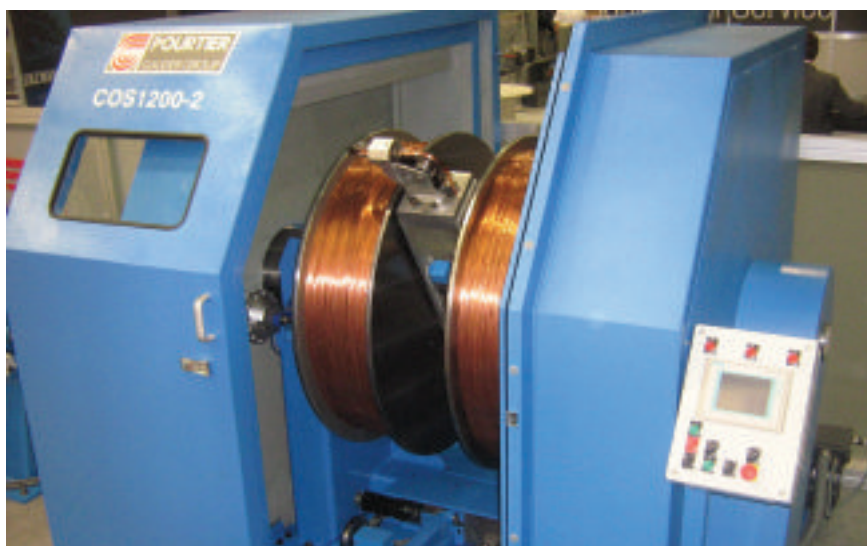
▲ COS 1200-37 multiwire concentric stranding line
