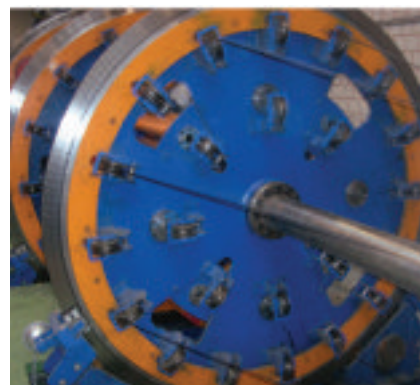
▲ Rim with 16 wires on the outer ring and eight on the inner rings
