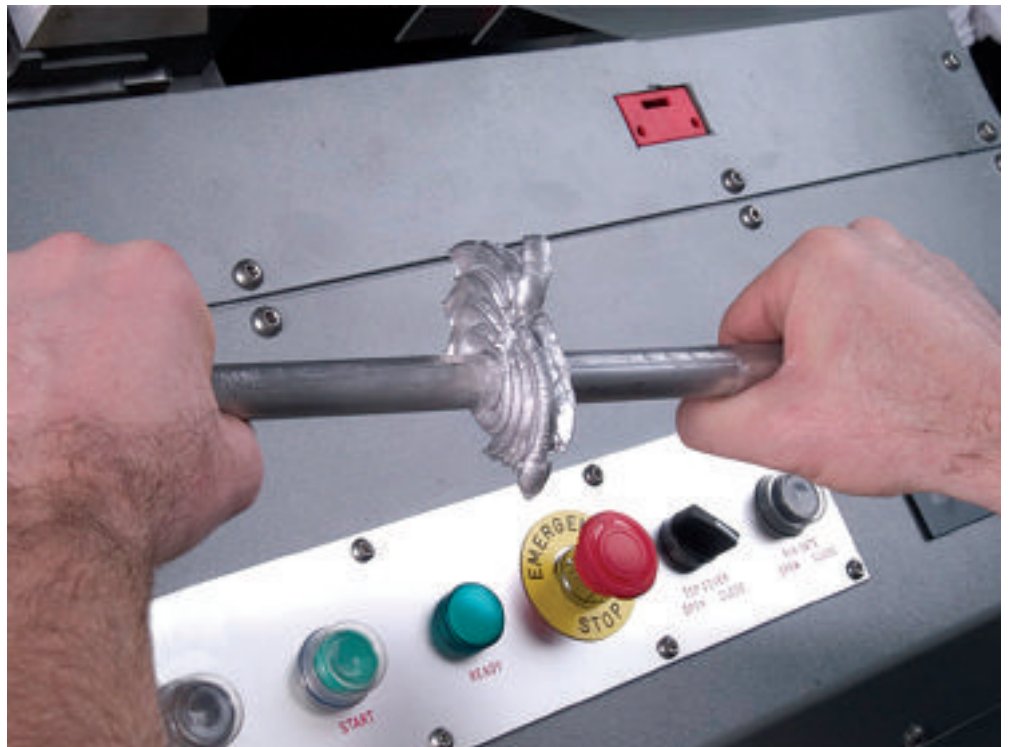
▲ The cold weld process creates a permanent bond stronger than the parent material
