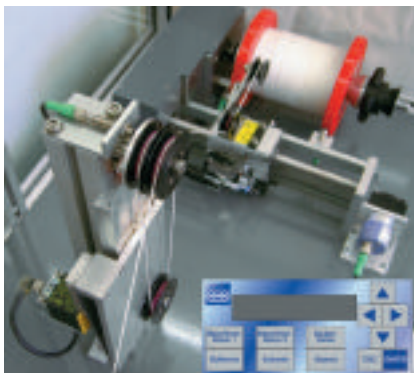
▲ AVS, automatic winding width control from Joachim Uhing
