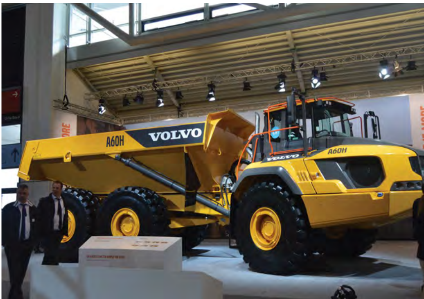
The new 55t capacity A60H is the largest machine to be built by VolvoCE
