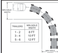
Minimum Aisle Width 8 feet (up to 3 Trailers)
