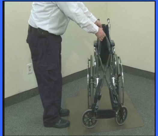
Lift up on the seat fabric and push in on the back fabric to collapse wheelchair frame.
