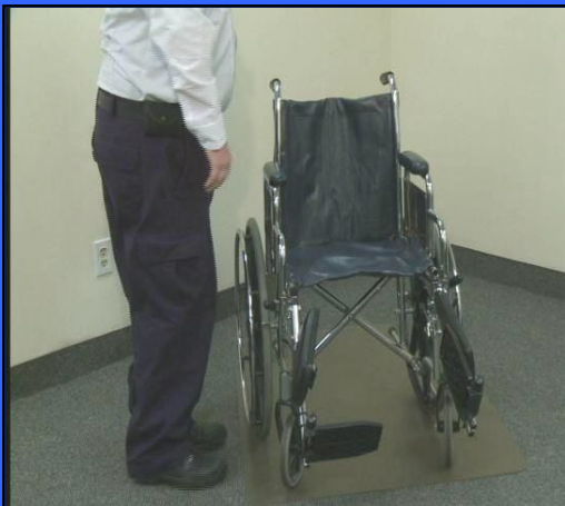
Continue pushing until the crossbar is completely deployed and the chair is fully open
