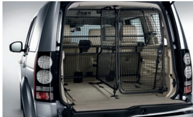
Cargo Divider EOH500040 Separates luggage space into two protected sections. Lockable outer gate on one side. Must be fitted with Cargo Barrier. Not compatible with standard Loadspace Cover.**
