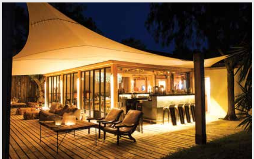
Warm white 5 W LED downlights illuminate the columns to create bounce light off the floor. This, with the under-counter strip lighting at the bar, makes a lively space for evening drinks.
