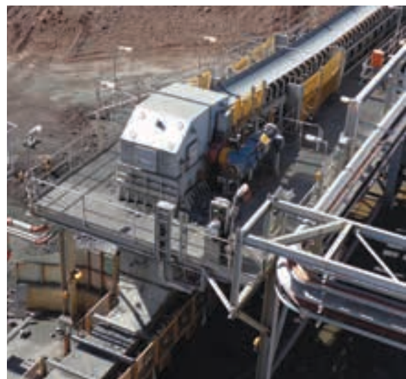
The Weba Chute System is a custom engineered transfer point solution designed to address the numerous issues plants face with material movement.
