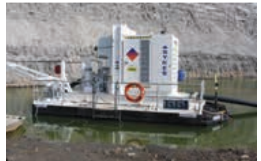
The Sykes Xtra High Head pump range caters to the arduous demands of the mining industry and all models have the ability to operate unattended at high discharge heads.
