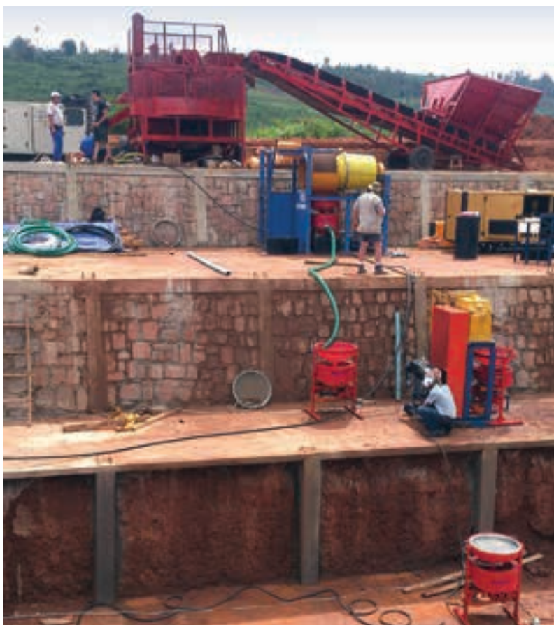
Small scale RG30 and GoldKacha for cassiterite recovery (cassiterite is the main tin ore).
