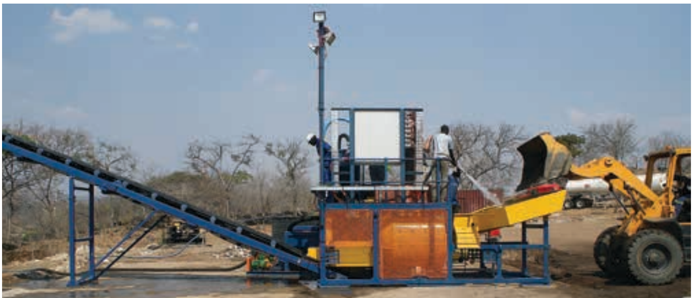
Below: An RG100 10 t/h scrubber wash plant.
