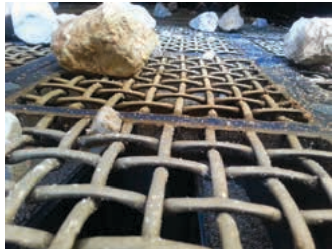
Modular polywire screen panel in a silica application.
