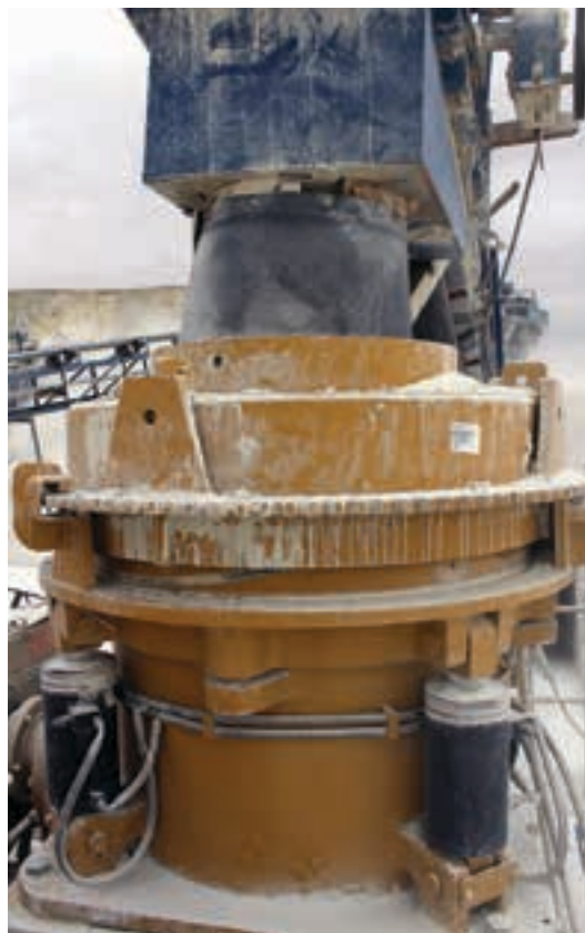
Trio TC36 short head cone crusher in a tertiary crushing application.
