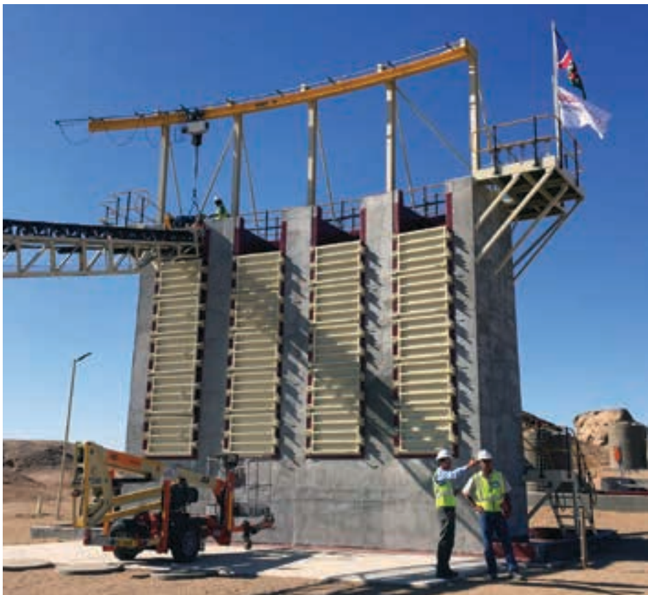
The Etango heap leach demonstration plant showing the leach cribs (photo: Bannerman Resources).
