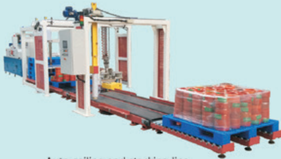
Auto coiling and stacking line
