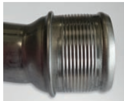
Grooves rolled between the beads from outside to inside
