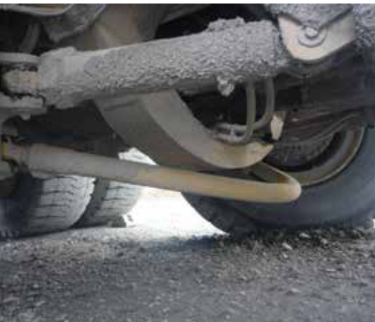
Figure 7: Bent tie bar as a result of poor road quality.
