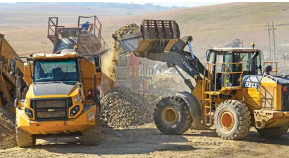
A Bell L2106E loads one of three pre-owned B30E trucks that Transkei Quarries added to its fleet earlier this year.
