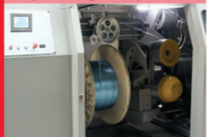
2 steps : Cabling line ("Quali2Twist")
