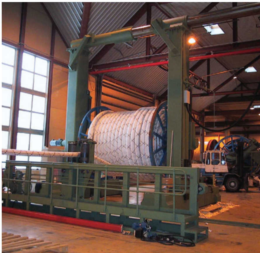
○ Tethering rope coiling system with a capacity of 118Te, suitable for rope, umbilical and cable coiling
