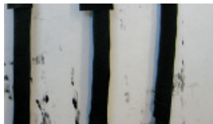
▲ Figure 7: The retention of an indicator flag of an EL-1392B cable upon 1061 cable flammability test
