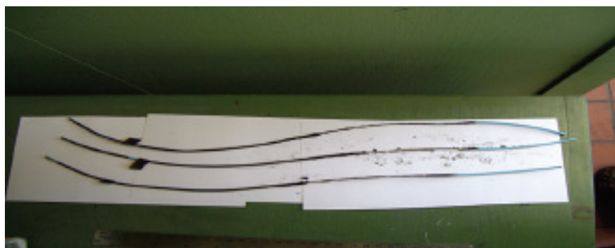
▲ Figure 6: The retention of an indicator flag of EL-1392B wire upon 1061 flammability test
