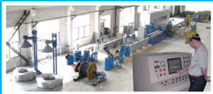
Continuous Aluminum Cladding Production Line for AS Wire, OPGW and Cable Sheath
