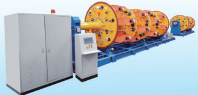
Planetary Cage Type Twisting Machine(Φ300/Φ400/Φ500/Φ630)
