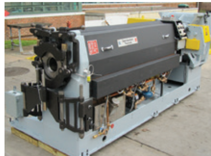
○ A rebuilt 150mm (6") Davis-Standard rubber extruder
