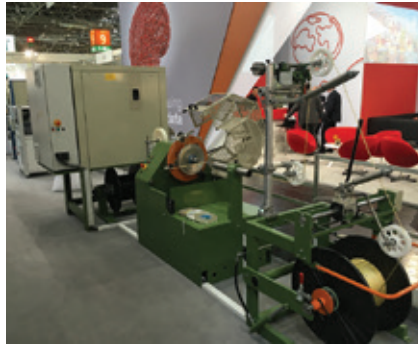
○ Improvements on the optimised braiding and taping line
