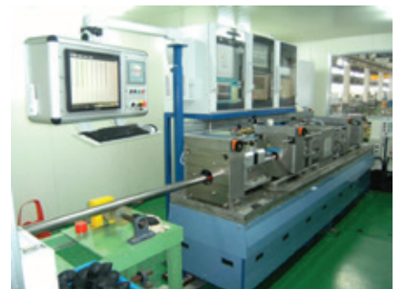
○ Complete titanium tubes inspection by UT and ET
