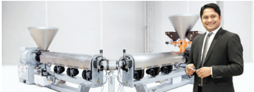
○ Solar cable co-extrusion from RosendahlNextrom
