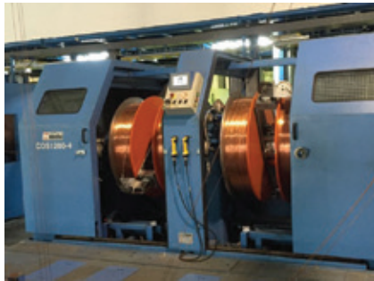
○ A power regenerative high speed concentric strander module of four reels with three wires each (Pourtier COS 1200-4)
