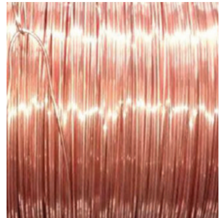
○ Plasma treated copper wire
