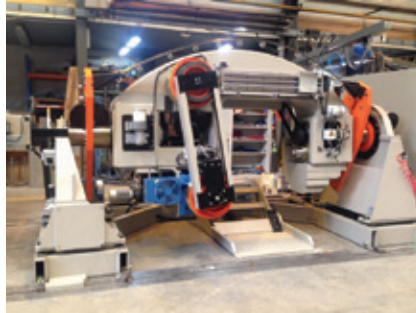
○ A large double twist stranding/laying-up machine (Setic TC 1250-4M)
