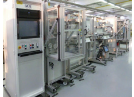
○ Optical fibre colouring from Medek & Schörner
