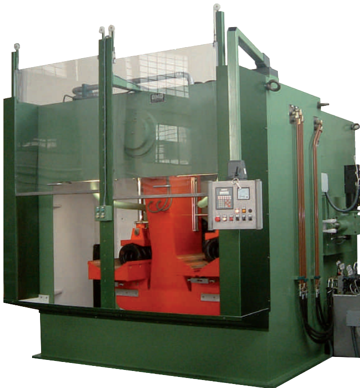
▲ The Series H150 traditional pendulum grinding machine
