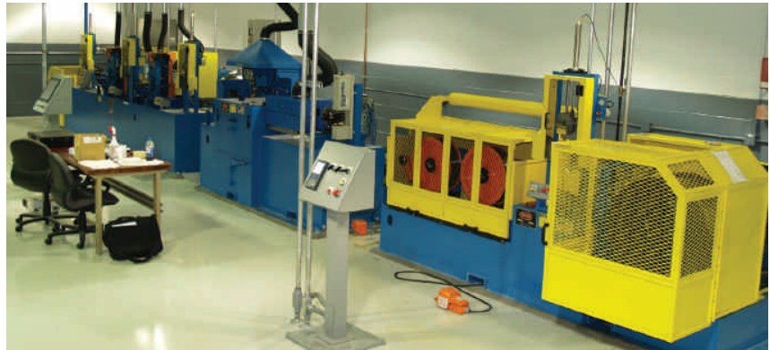
▲ Fenn Technologies' new wire flattening and shaping line
