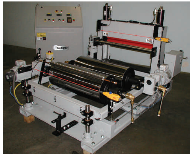
▲ The new 30" (750mm) cast film take-off
