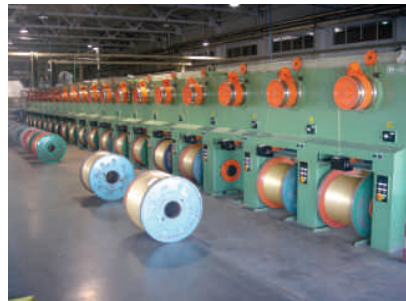
▲ Spool take-up frame with double accumulation capstan for non-stop operation
