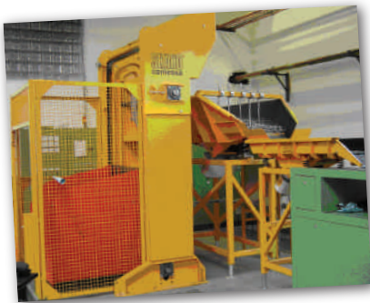
▲ Skako Comessa's lift-and-tipping system – Tilde
