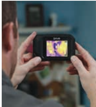
A FLIR C2 being used to locate an insulation void in a bedroom wall.
