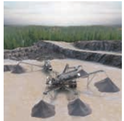
The combination of the Metso NW106 primary jaw crushing plant and the NW220GPD secondary cone crushing plant with a large dual-slope screen requires no foundations and has been designed to be “easy and safe” to operate and maintain on site.
