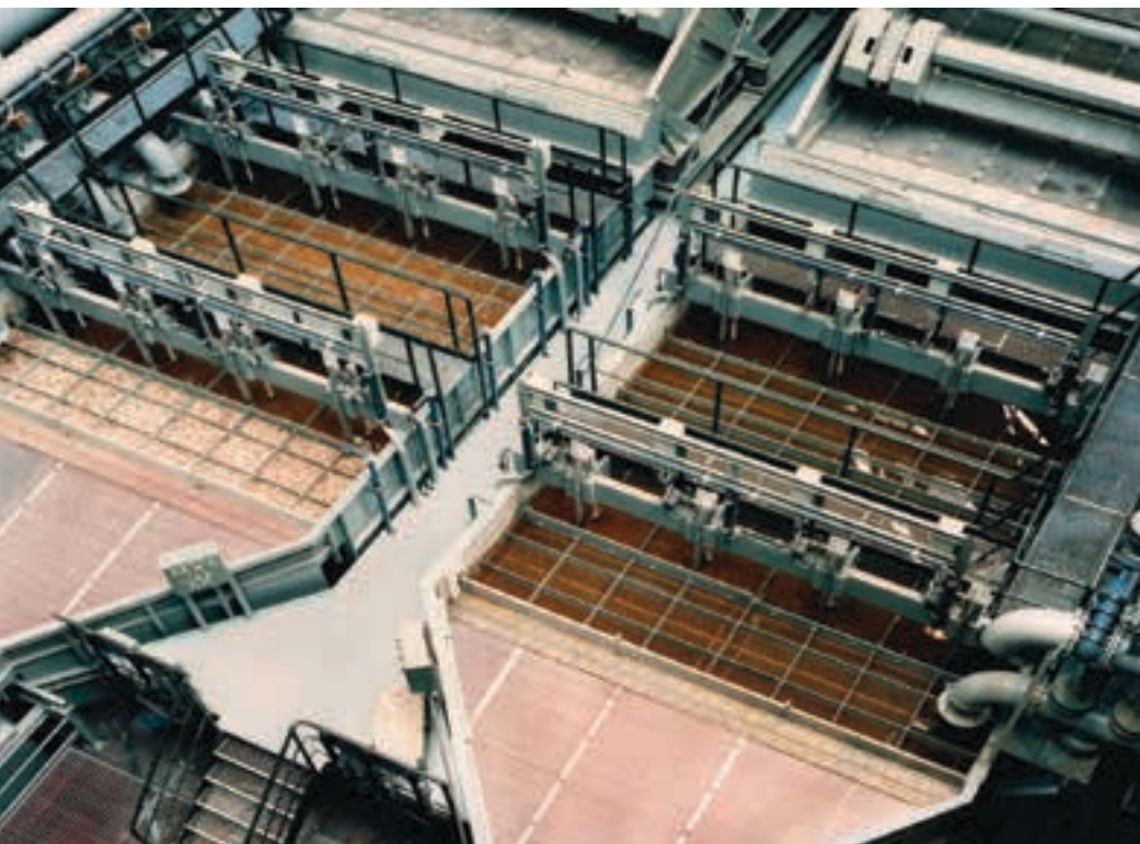
BATAC® jig technology has excellent separation accuracy, is relatively small in footprint and has a comparatively low capital cost.
