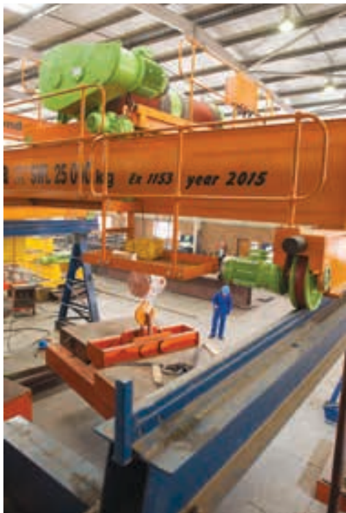
Load testing on one of the two 25 t headgear cranes manufactured by Condra for Mopani Copper Mines' Sinclinorium shaft.
