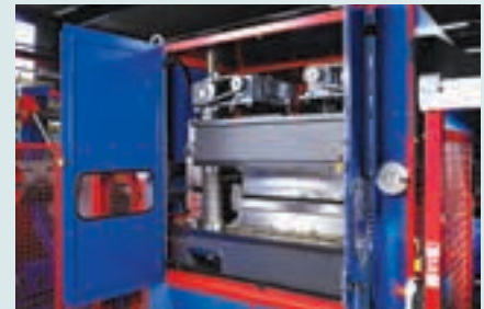
The type TSD 4-1600 press boasts a coil line with a fine levelling machine from Schuler.
