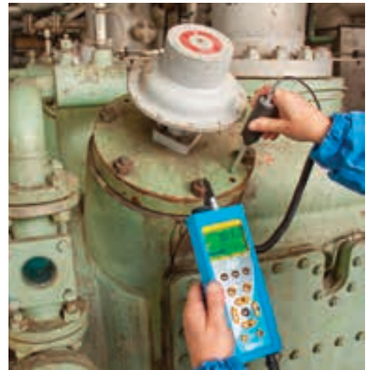
Ultrasonic detectors can locate and quantify compressed air, gas and steam loss to leaks and faulty traps, passing process valves, cavitating pumps, over lubricated bearings and more.
