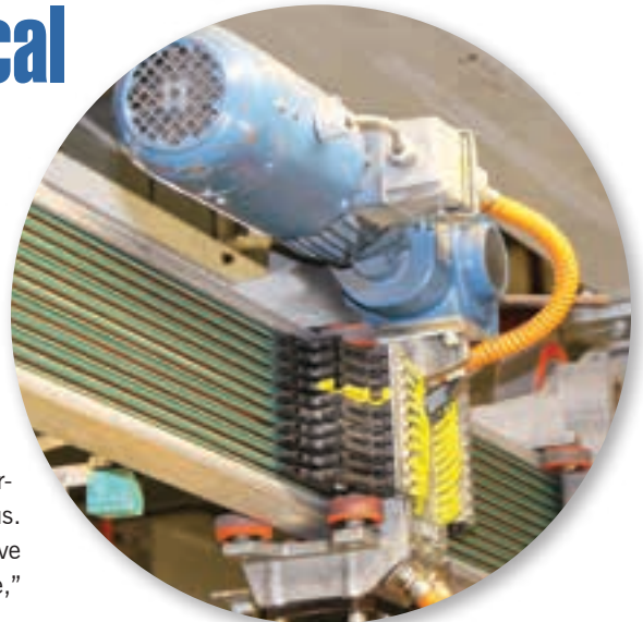
The DMS uses polyurethane tyres to prevent metal-on-metal flaking.
