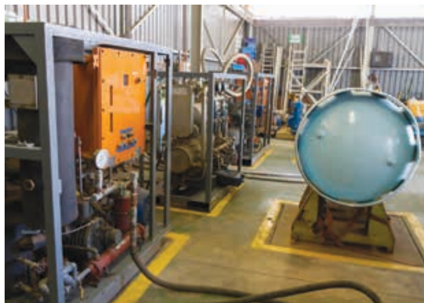
The Zugibeast is a high-speed decontamination unit used to extract contaminants from refrigerants.
