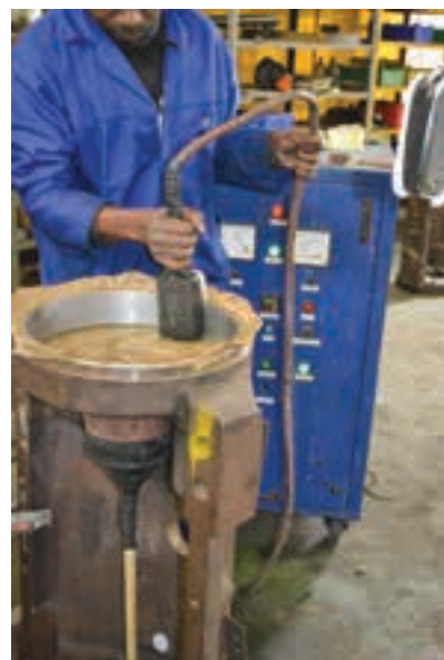
A surface being selectively electroplated using the brush on process. Electrolyte is passed through the positively charged anode wrapped with a soft, felt-based absorbent cover material. While being brushed around the surface being coated, metal atoms are deposited on the surface of the component, which is negatively charged (cathode).
