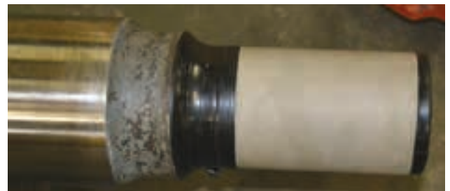
The journal-bearing surface of a shaft coated with a nickel cobalt hardened layer.
