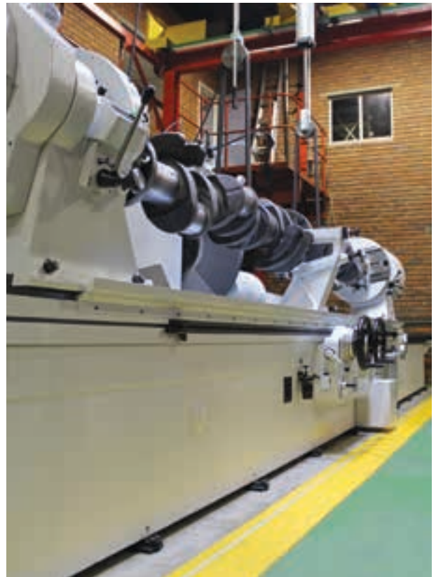
The largest crankshaft grinding machine in Africa is hard at work at Metric Automotive Engineering.
