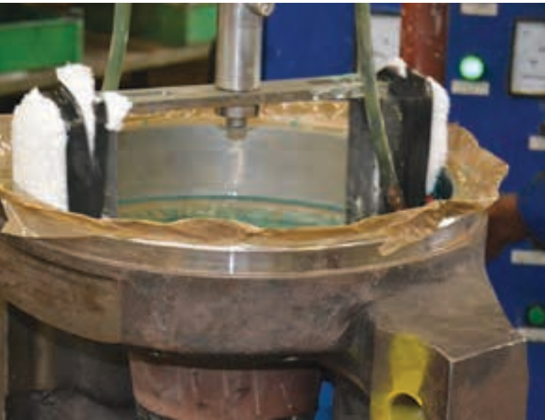
After starting the process manually, the plating is mechanised by attaching the two plating shoes to a rotating beam. The total electrical energy in kWh is used to determine the coating thickness for a given area to a thickness accuracy of better than 99%.
