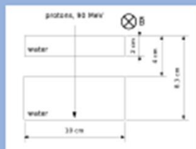
Simulation setup for the calculation of proton dose distribution in the presence of a magnetic field in a homogeneous water phantom (3 and 4 water phantom with an air gap). Note that in situation (3) the Bragg peak is located at the distal water-air interface.
