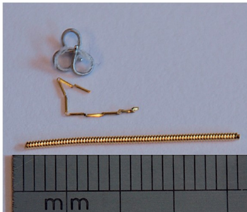
Figure 1. Photo showing the complex helical platinum marker (top), the Gold Anchor™ marker (middle) and the Visicoil™ gold marker (bottom).
