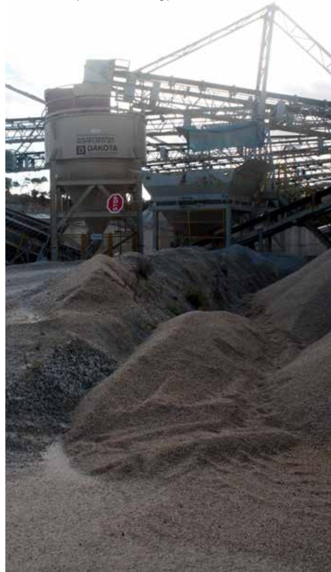
The Dakota air separator and washing plant.
