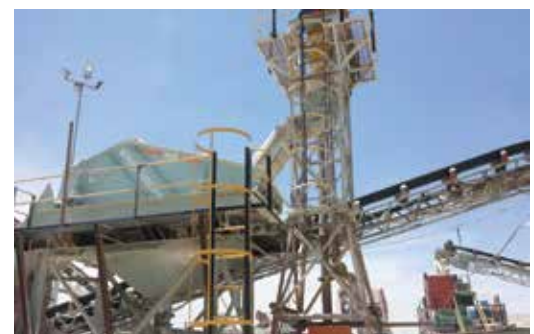
A Cavex CVX cyclone and Enduron dewatering screen optimising production in a crushing application.
