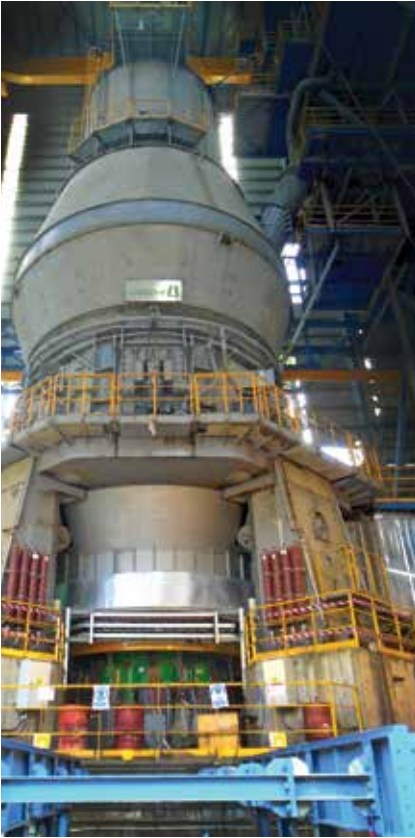
The Loesche LM 70.4+4 CS is designed for a capacity of over 370 t/h.
