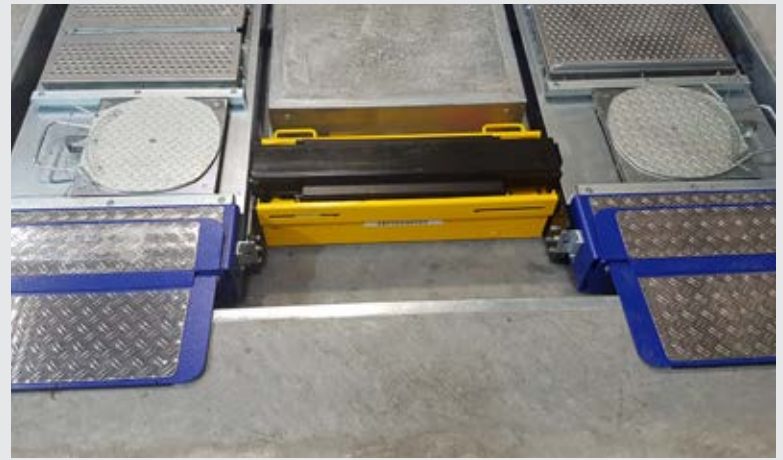
Sunken Jacking Beam
