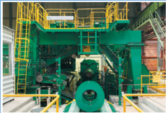
Coil handling equipment
