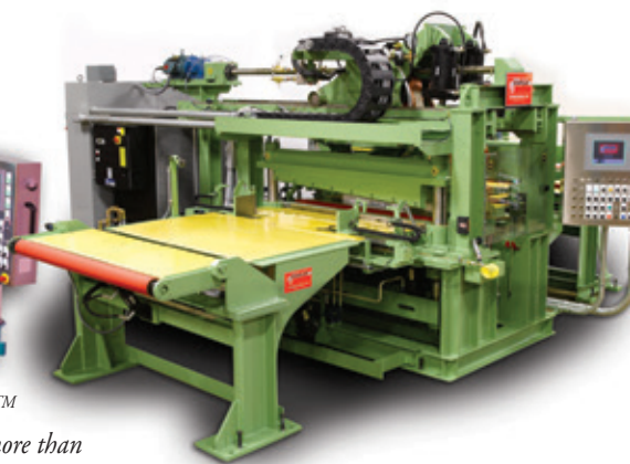
NB Overlap Resistance Zipwelders™ produce fast, high strength welds.
