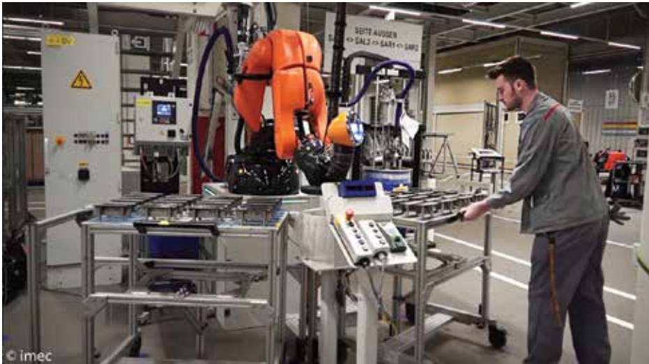
Fig 2: The cobot developed for Audi can be operated using hand gestures and has a screen in the form of a face to communicate with the worker.
