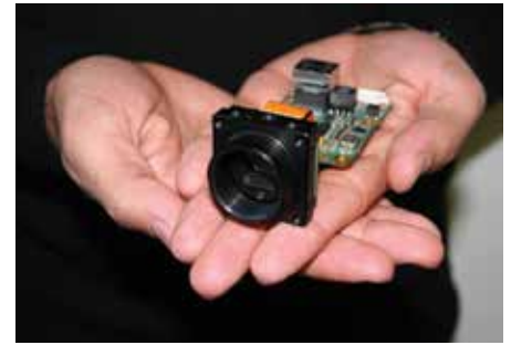
Figure 1: Embedded vision systems typically combine a camera, processing device and interface
