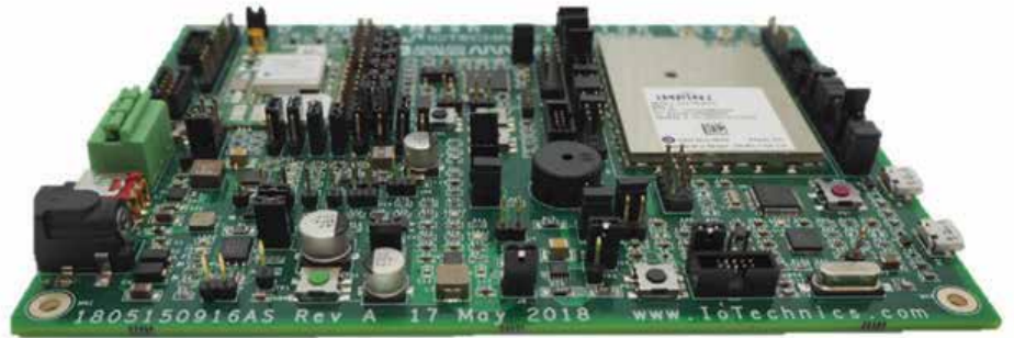
Image 2: RFID reader solution
