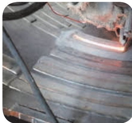
Figures 12: Field tests. Cladding of a reactor shell with RECORD EST 625-1 LD.
