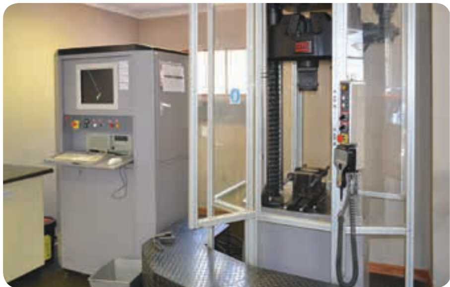
Above: SAIW's fully automated MTS Criterion tensile testing machine.
