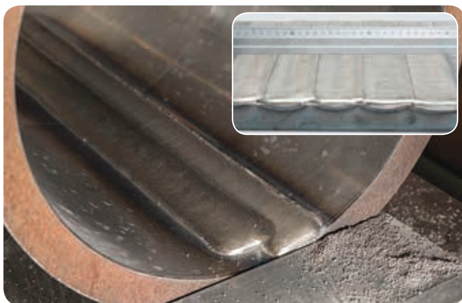
Above: Cladding using voestalpine Böhler Welding's advanced strip cladding process enables thin layer Alloy 625 deposits that meet iron (Fe) content requirements.
