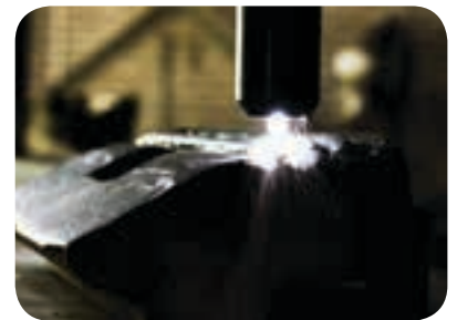
PTA clad hardfacing offers the ideal solution for applications where severe impact and corrosion are prevalent.
