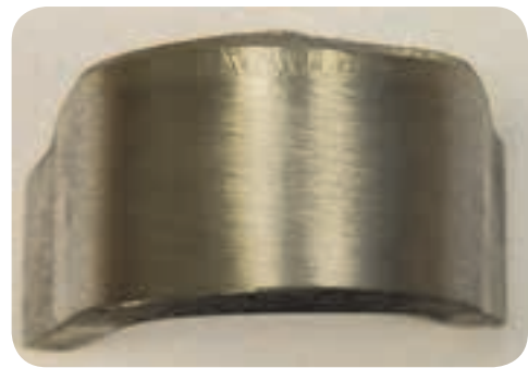
Figure 4: Side bend test. Cladding deposit produced with RECORD EST 625-1 after PWHT at 670 °C for 24 hours.
