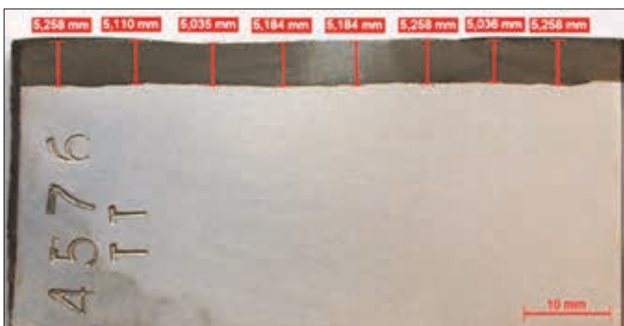
Figure 7: Bead profile of cladding with RECORD EST 625-1 LD, with Fe < 7% scenario.
