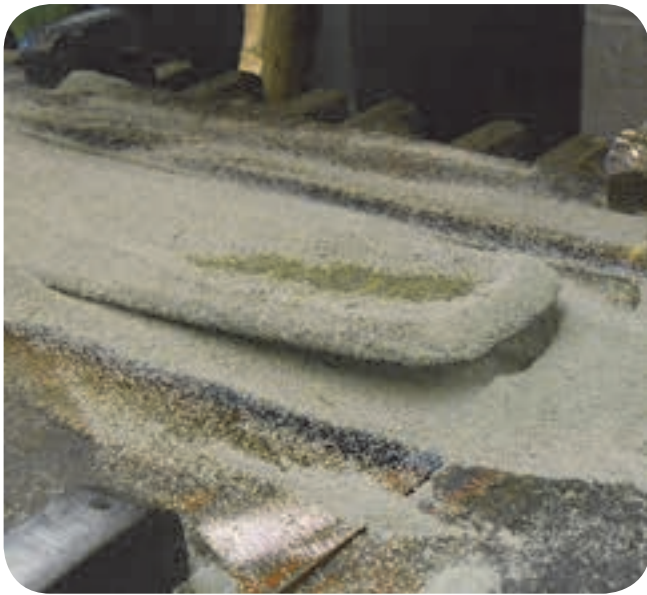
Figure 10: Advanced electroslag cladding with RECORD EST 625-1 LD showing the self-releasing slag.
