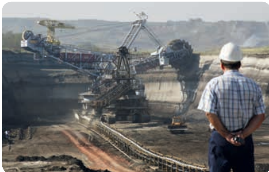
The buckets on a bucket wheel reclaimer will typically be subjected to abrasive and impact wear.
