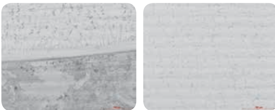
Figure 9: Micrographs. RECORD EST 625-1 LD cladding after PWHT at 670 °C for 24 hours. From left to right: fusion line area, middle of the bead.
