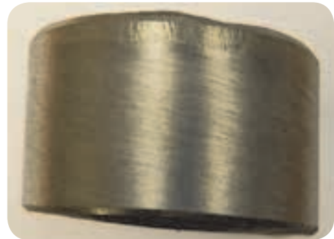
Figure 5: Side bend test. Cladding deposit produced with RECORD EST 625-1 LD after PWHT at 670 °C for 24 hours.
